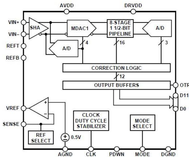
Figure 5 A/D Conversion Unit Functional Block Diagram
