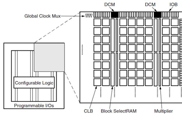
**Figure 3 Programmable Logic Unit Architecture Overview**
