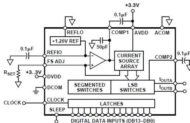
Figure 6 D/A Conversion Unit Functionnal Block Diagram
