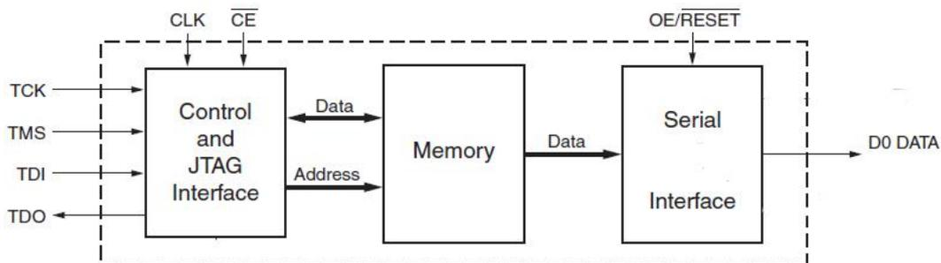
Figure 4 Configuration And Memory Unit Block Diagram
